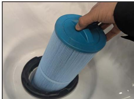
When removing the filter cartridge, you may remove the filter by turning it counter clockwise. The filter must be removed gently to not damage the threaded fitting inside of the filter canister.
